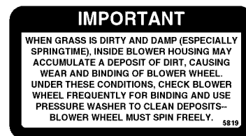
Top of Blower Housing (5819)
