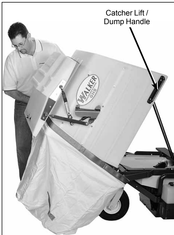
Dumping Catcher into Dump Bag
