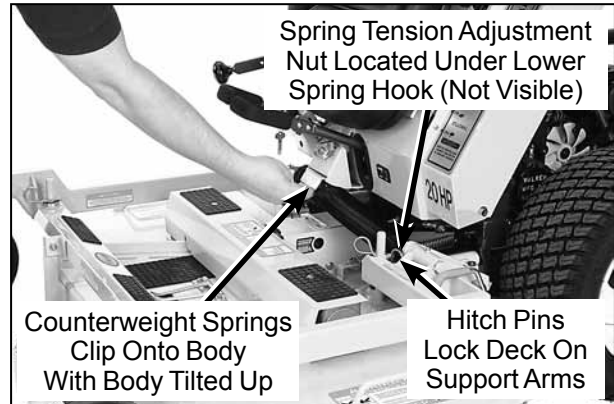
Deck Counterweight Spring Installation
