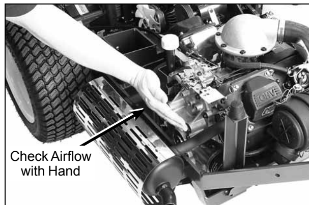
Cooling System Airflow
