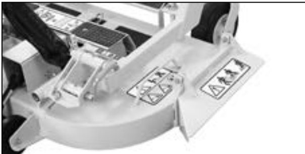
Side Discharge Deflector Shield in Lowest Position
