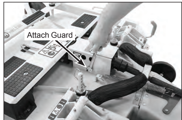
PTO Shaft Guard Installation
