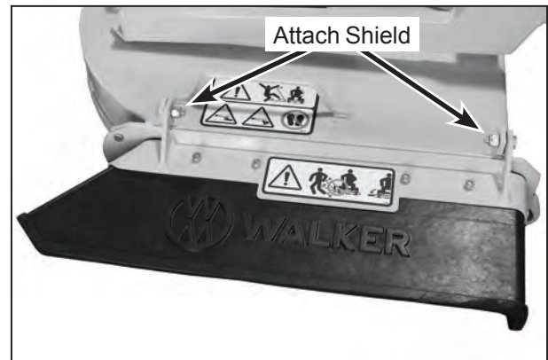
Discharge Shield Installation on Side Discharge Deck
