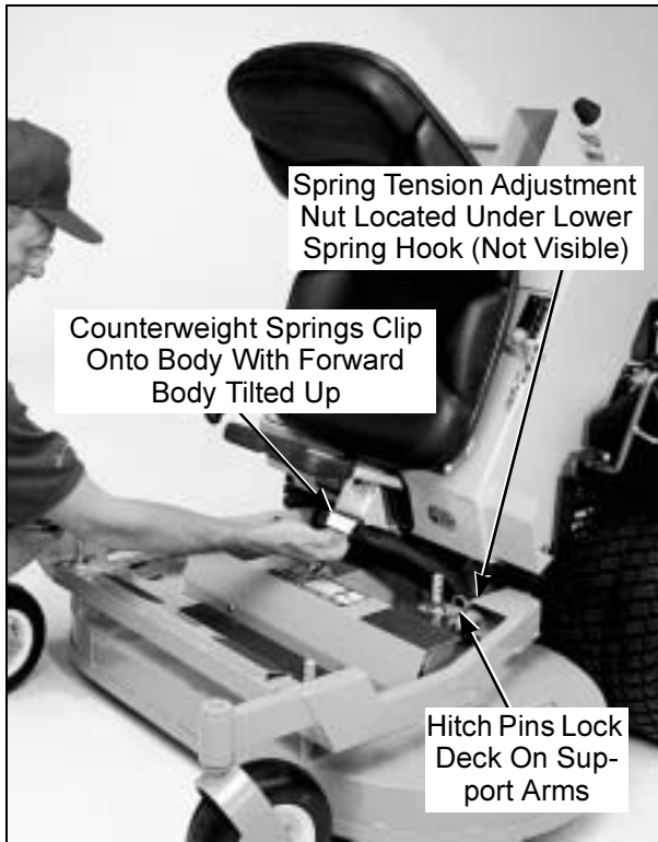
Deck Counterweight Spring Installation
