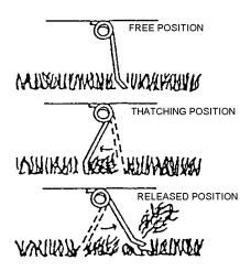
**MAINTENANCE** - The Walker Lawn Dethatcher is maintenance free. However, as with any steel product, given enough time, it can rust. For rust on the tines, apply a light coat of oil. For rust on the tray or mounting brackets, simply sand lightly and coat with an enamel.
