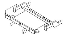
1/4 02/23/96 Revision B Dated 03/28/03 Revision C Dated 02/29/08 **ADJUSTMENT** - Loosen the four (4) nuts on the sides of the tray mounting brackets. Adjust the tine tray to locate the tine ends approximately 1/2" above the flat surface when in the free position and touching the flat surface when pushed back. Tighten four (4) nuts.
