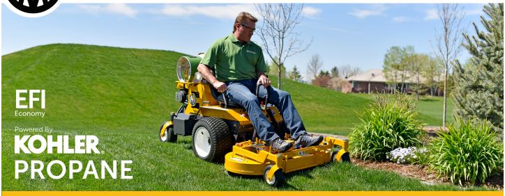
The B25p features a breakthrough Kohler EFI propane engine delivering power and performance from a clean fuel. With a 33.5 lb tank the B25p provides extended hours of operation for commercial or municipal operations.
