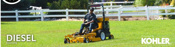
For discerning operators, the H24d delivers an impressive package. Featuring a Kohler KDW1003 diesel engine with 1028 cubic centimeters of displacement, the H24d provides consistent power and smooth, quiet operation. The self-cleaning radiator, 9.4 gallon fuel capacity, and Grammer suspension seat allow for comfortable extended operation. The standard utility bed and optional add-ons make the H24d a versatile, year-round performer.
