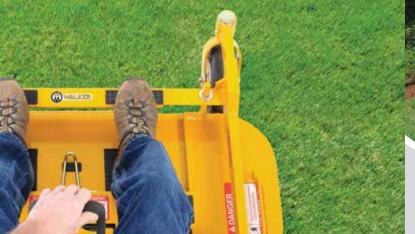
The compact Walker fits in places most other commercial mowers can't, quickly maneuvering into each nook and cranny to finish the job in one pass. Forward/reverse, zero-radius turns, and braking are accomplished by lightly pulling the steering levers while the FSC adjusts and holds forward speed.
