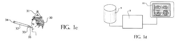
Figures 1a–1d depict schematic views of computer-assisted microsurgery equipment. *Id.* at 3:59–60. As illustrated in Fig. 1a, the equipment includes articulated tool support 1, one end of which (i.e., base 11) is integral with fixed reference frame  $R_c$  (e.g., the ceiling of the operating room). *Id.* at 4:5– 7. Articulated tool support 1 comprises trihedron 21 made up of an assembly of four light points (e.g., electroluminescent diodes) 22–25. *Id.* at 4:23–26.
