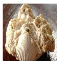
After four days, water is poured on the blocks, which now have changed to brittle white chunks show-casing seashells from centuries past. The pieces are ground down and sifted into a fine powder that we know as lime in English, in Spanish it is called "cal."
