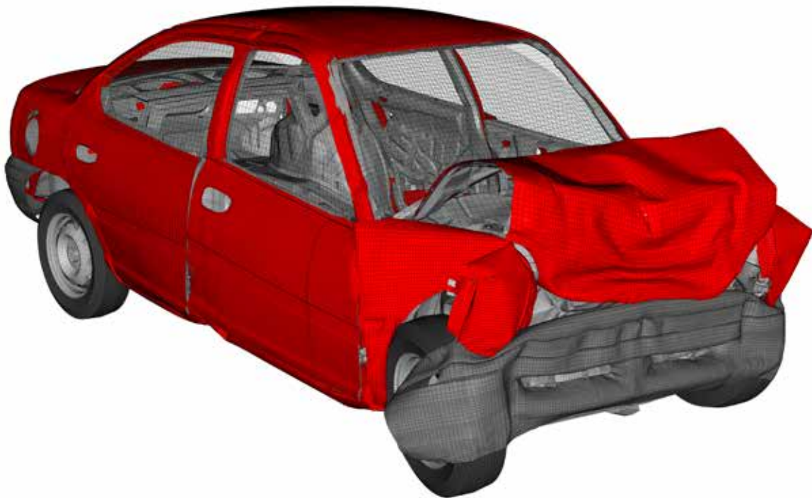
Figure 7. Modified Chrysler Neon* model (1 million elements) used in RADIOSS* crash simulation benchmark testing.
