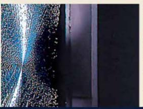
LAMINATED GLASS MAY CRACK UNDER PRESSURE, BUT TENDS TO REMAIN INTEGRAL, ADHERING TO THE VINYL INTERLAYER
