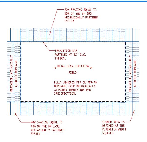
WITH THE EXCEPTION OF THE TRANSITIONAL BAR DIVIDING THE FULLY ADHERED AREA FROM THE MECHANICALLY ATTACHED AREA, ALL ATTACHMENT MUST BE INSTALLED PERPENDICULAR TO THE METAL DECK FLUTE ORIENTATION.
