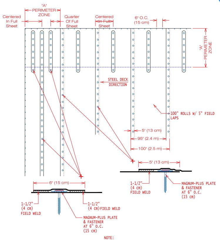
DIMENSION "a" SHALL BE DETERMINED BY CURRENT ASCE7 OR FM APPROVALS CRITERIA FOR DETERMINING WIND ZONE WIDTHS. SEE FIBERTITE DETAILS FTR-ASCE7a THROUGH FTR-ASCE7d FOR ILLUSTRATIONS PERTAINING TO CALCULATING ROOF WIND ZONE.
