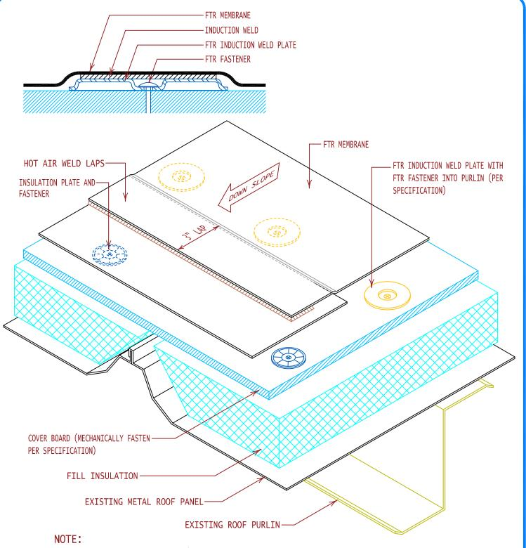
REFER TO DETAIL FTR-IWS1 FOR PROPER PLATE SECUREMENT TO ENSURE MAXIMUM MEMBRANE TO PLATE BONDING. WHEN INSTALLING MULTIPLE LAYERS OF INSULATION, ALL END JOINTS SHALL BE STAGGERED.
