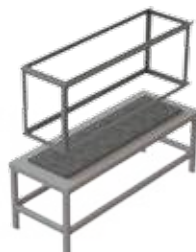
Lower frame over mounting subpanel
