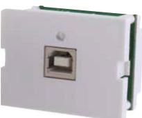
Hubbell's USB 110 Extender transmits 2.0 High Speed signals over one solid, unshielded, twisted-pair (UTP) cable, allowing data device to be located up to 100 feet away from a digital source. The USB extender is ideal for extending control to projectors, smart boards, flat screens and other data devices. It also supports high speed applications such as cameras, document transfers, and video conferencing.
