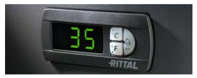
The internal temperature of the enclosure should always be set to +35°C. There is no technical justification for setting the temperature any lower. If the temperature inside the enclosure is lower than that, e.g. +15°C, condensation will be significantly increased. The parts and components will also become sub-cooled and form condensate after the cooling is switched off or the enclosure door is opened.
