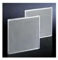
If the air is oil-contaminated, use metal filters. These separate the oil condensate from the air and can be cleaned with appropriate detergents.
