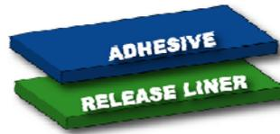
TF1573 is an unsupported, permanent PSA transfer film. A specially formulated solvent acrylic adhesive designed to promote excellent wet-out to a variety of substrates including low surface energy plastics.
