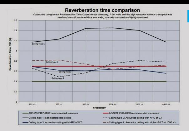
The table above illustrates this point: wider frequency analysis approach is important when selecting an acoustic material. Ceilings 2, 3 and 4 all use a material that has a single number sound absorption rating of 0.7, and yet the results couldn't be more different.
