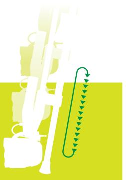
**tilt** Tilt allows you to keep the center of the pipe in the center of the video frame as you zoom:
