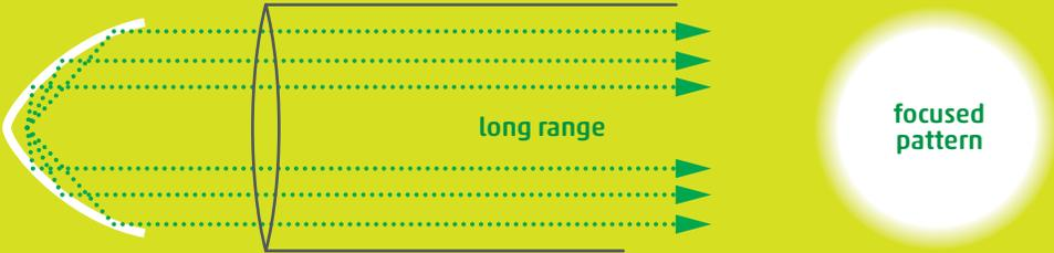
parabolic lamp reflector (collimating)
