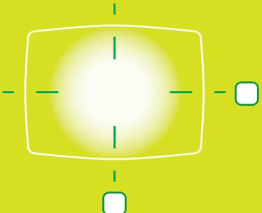
**intensity** The usefulness of lamp intensity depends entirely on the system's focus and alignment, as well as the camera's sensitivity. For that reason empirical data (like wattage or luminous flux) means very little. You should instead rely on your perception. See how many segments you can count as you zoom toward the far end to estimate total range.
