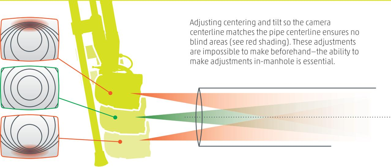
Adjusting centering and tilt so the camera centerline matches the pipe centerline ensures no blind areas (see red shading). These adjustments are impossible to make beforehand—the ability to make adjustments in-manhole is essential.
