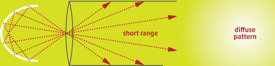
elliptical lamp reflector (non-collimating)
