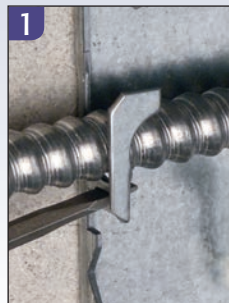
1 Insert screwdriver through slot.
