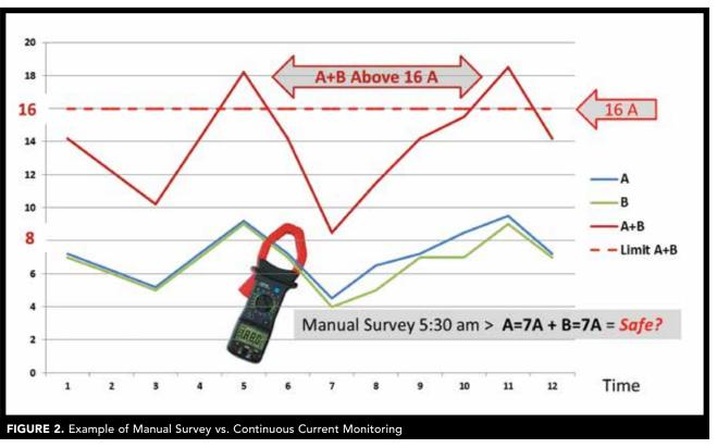
Example of Manual Survey vs. Continuous Current Monitoring
