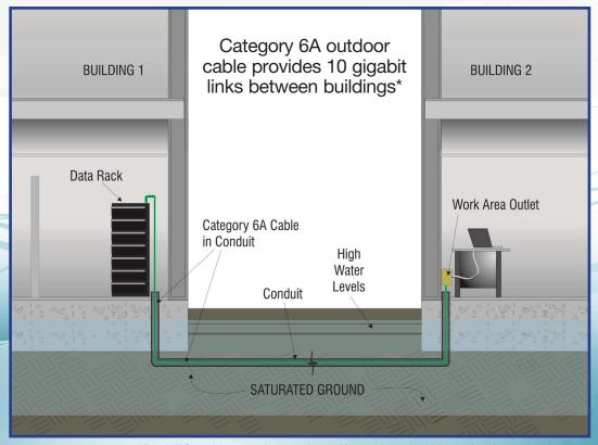
\*Per NEC, cable must be terminated/transitioned within 50 ft. of entering building.
