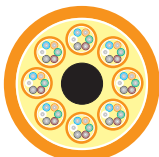
48-fibers (8 tubes of 6-fibers)
