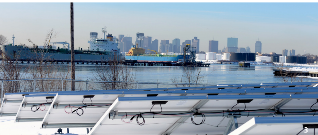
2 & 3 At Fraunhofer CSE's Revere, MA outdoor testing facilities, modules are exposed to both winter and marine conditions.
