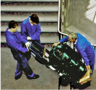
PowerMate® powers loads up/down stairs, on/off vehicles or loading docks and moves loads across flat surfaces in a completely balanced position.
