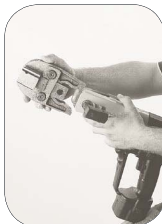
Place the jaws in the housing
