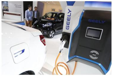
Fuel-sippers using 48-volt batteries get much of the benefit of full hybrid at a lower cost. Geely Automobile and other top Chinese car makers are lining up behind so-called mild hybrid cars that rely on an auxiliary 48-volt system to power some energy-intensive components and boost fuel efficiency. PHOTO: WU HONG/EUROPEAN PRESSPHOTO AGENCY
