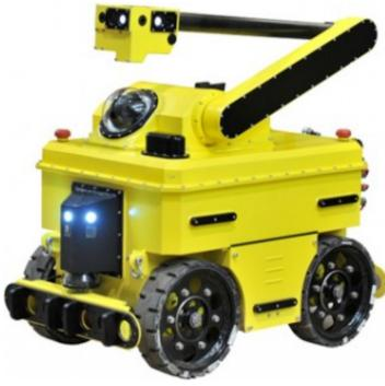
Shell and CMU's Sensabot is designed for on-site inspections.
