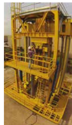
DTI Drilling Systems' riser tensioner system has been developed to reduce weight and space in the moonpool Source: DTI Drilling Systems
