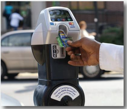
The new parking meter features include; environmentally friendly solar power, high contrast displays for viewing, multiple payment options of credit/debit card and coin, and an option to allow drivers to pay-by-cell phone in the future.
