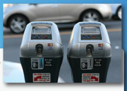
The new meters have been operational approximately 99% of the time, and they call for repair if they are vandalized or malfunction. If a Coin & Card meter needs service, it sends a wireless message to a technician, improving the efficiency of repair to return failed meters to service quickly.
