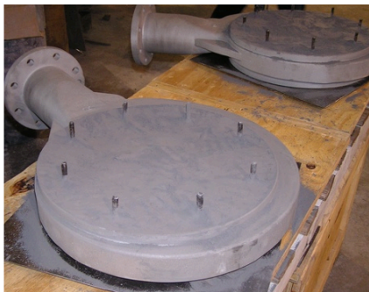
Wet Gas Scrubber Nozzles loaded for Boronizing
