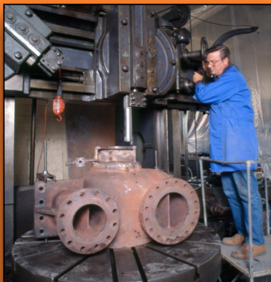
Machine Shop Capable of Turning 68" Diameter Parts for Repair
