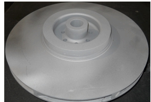
Boronized Impeller for Refinery FCC Service
