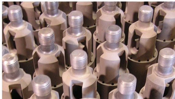
Boronized Plungers used in Oil Production
