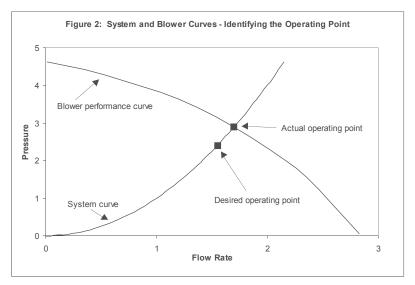
best served by selecting the blower that . delivers the desired performance with the least amount of input power. Typically, the most efficient blower is the one where the system resistance curve intersects the blower curve at approxi- able for powering the blower? mately the middle, i.e., half the maximum flow rate.
