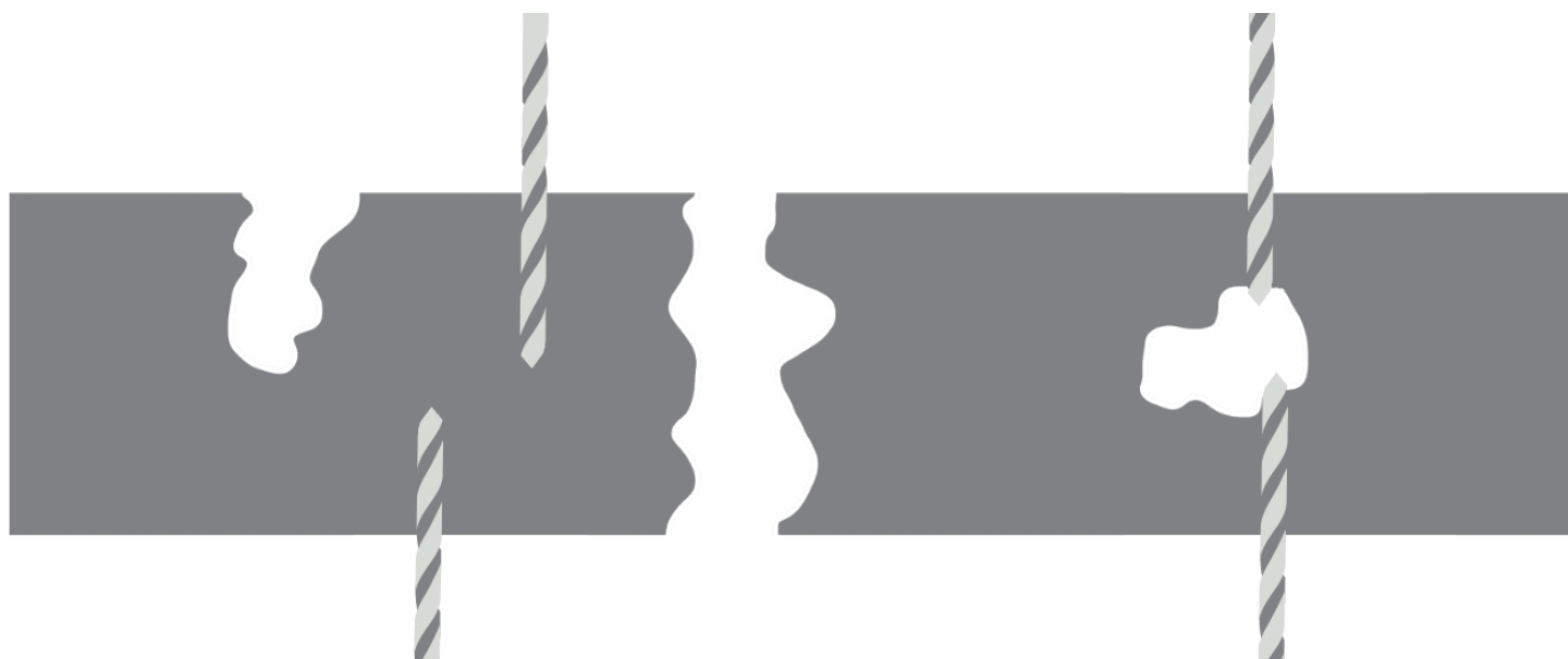
Figure 5: Porosity can be opened during final machining, causing previously undetected leak paths.
