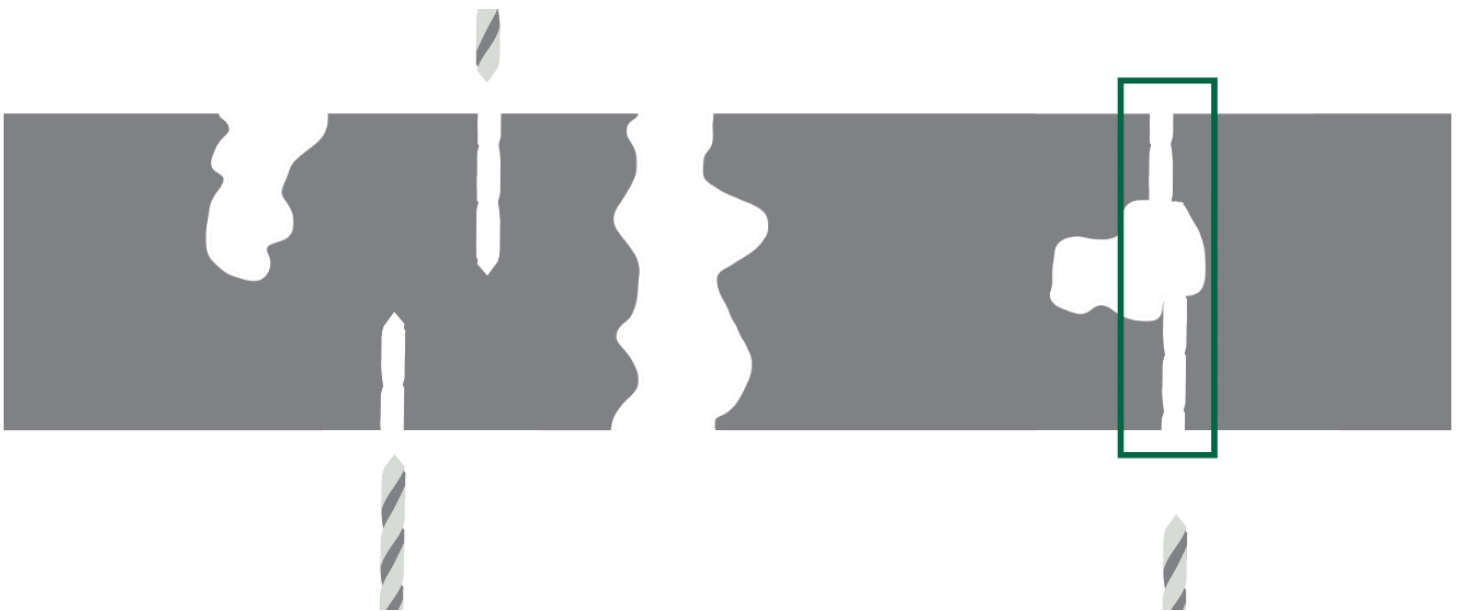
Figure 6: Machining can cause new inter-connected porosity
