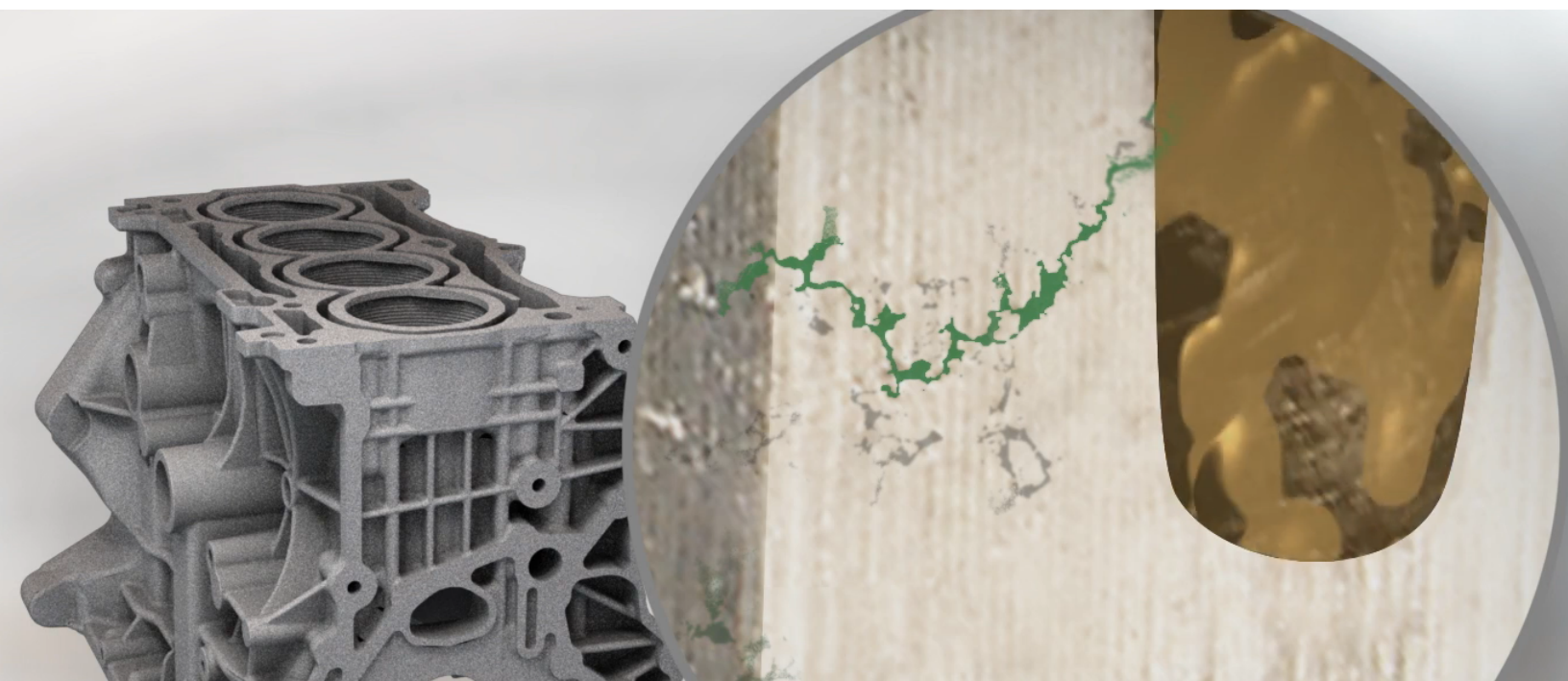
Figure 9: Vacuum impregnation seals the porosity, while any sealant on the surface are washed away.
