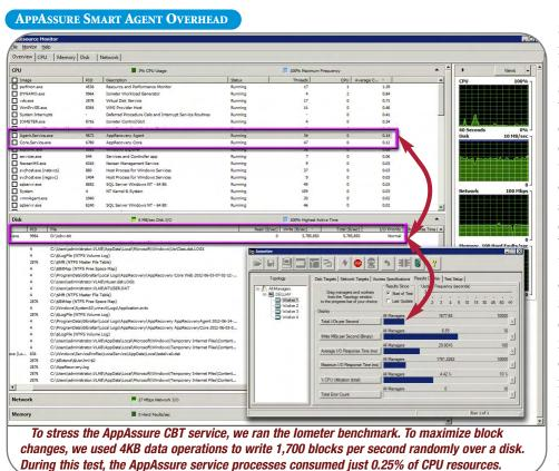
The AppAssure Smart Agent places a filter driver between the Windows file system and the Windows kernel to capture block-level changes on the underlying logical disk volume associated with data changes in files made by applications. Using the filter driver, AppAssure Smart Agents on client systems log meta data about disk-block changes for each logical disk. During a backup, the agent utilizes the meta-data logs to send an AppAssure Core server all of the
