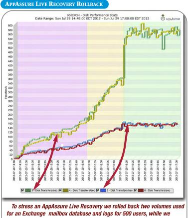
for an Exchange mailbox database and logs for 500 users, while we simultaneously ran Jetstress. During the process, Live Recovery allowed Exchange server to successfully respond to all Jetstress requests. The I/O response rate increased slowly until 65% of the data had been restored, when both the response rate and rollback throughput rapidly increased.
