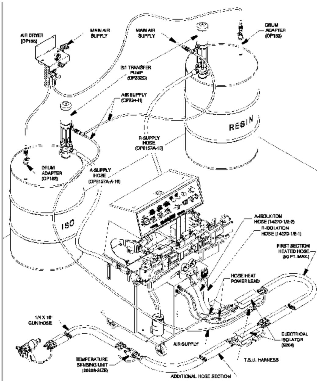
Typical spray polyurethane foam equipment setup
