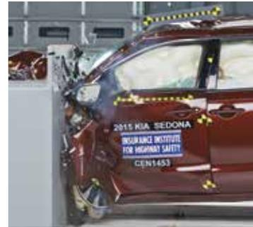
The doors of most late-model vehicles automatically lock when the vehicle is in gear or reaches a certain speed. In some cases, the feature can be disabled by the consumer. For those vehicles, the Institute's policy is to unlock the doors for the test.
