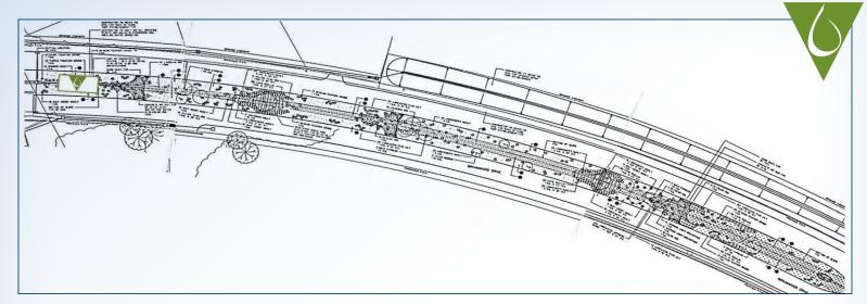
PLAN VIEW OF BIRNAMWOOD DRIVE: You can see in the small footprint of the FocalPoint Biofiltration System in relation to the remainder of the bioswale.
