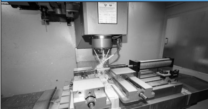
CLOSE TOLERANCE PISTON ROD MACHINING AFTER CYLINDER IS ASSEMBLED
