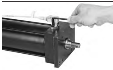
Bolt sensor to cylinder.
