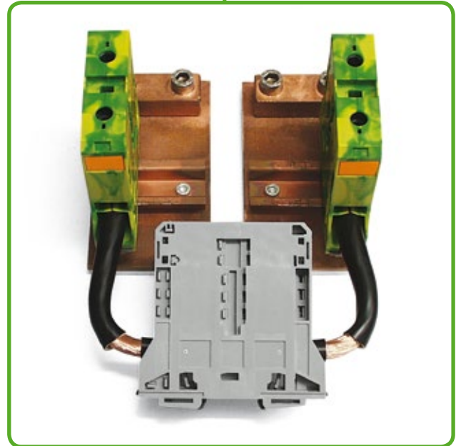
Test arrangement: "Short-Time Current Withstand Test"
