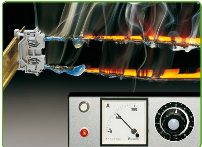
Test arrangement: "Short-Time Current Withstand Test"
