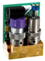
Common supply inlet and exhaust ports with manifold mount assembly. MPV2 accepts feedback signal from an F-Series flow transducer for closed loop flow control. Also accepts external feedback of pressure, vacuum or force. DIN rail, panel mount or up to 12 stations sub-base manifold mounting options available.
