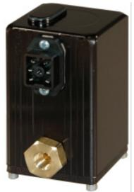
Analog monitor output is standard, select 0-10 VDC or 4-20mA. The dual loop design accepts feedback signal from a wide range of external sensors. The QPV2 accepts feedback signal from F-Series flow transducer for closed loop flow control. It also accepts external feedback of pressure, vacuum or force. Optional digital display is available.
