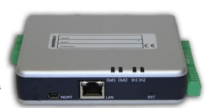
This is a compact DIN-rail or wall mount solution that enables analog sensors (voltage or current) to easily and transparently send real-time data to any node on the Internet or to a Cloud-based application. It also converts Ethernet to analog commands so analog controlled devices can be directly controlled from a computer or other Ethernet generating device. There are two analog puts for this function.
