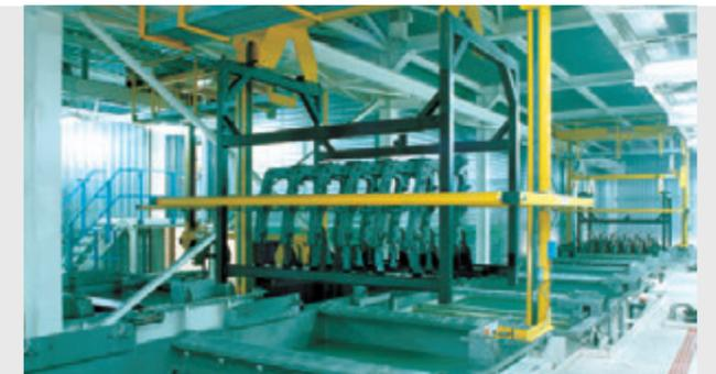
*Electrophoretic dip coating is supremely suited to prevent corrosion, and can be used in mass production as well as for single-size lots.*
