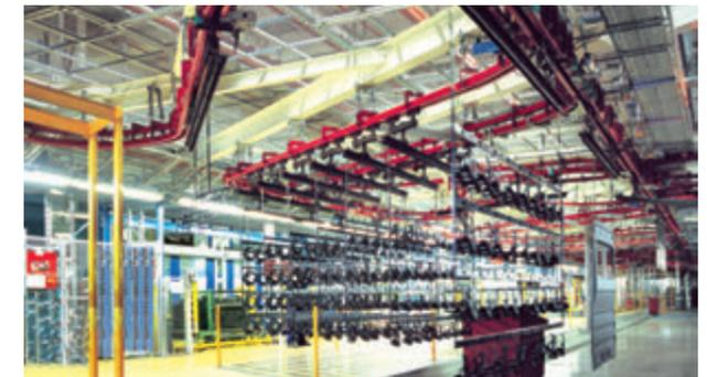
*Complex power & free conveyor system with numerous pick-up stations, interim storage and process destinations in the automotive industry.*
