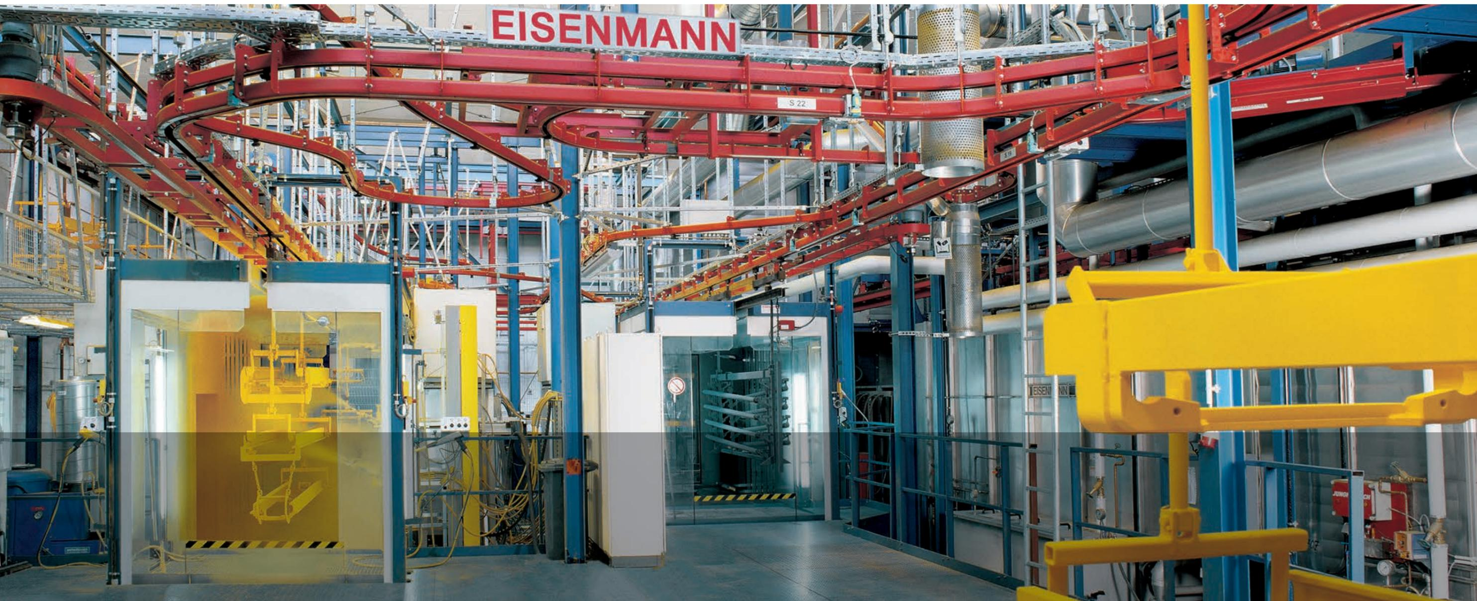
*Powder coating line with power & free conveyor for forklift components.*
