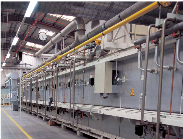
Zones with process-related atmosphere and temperature in a continuous kiln
