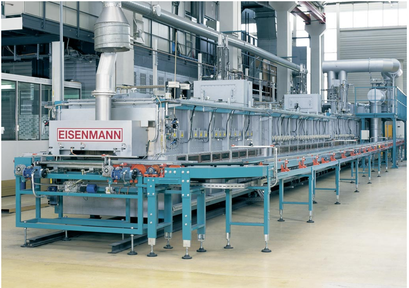
Roller hearth furnace for sintering process up to 1280 °C
