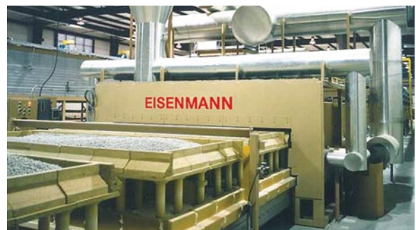
Calcination oven for catalyst material
