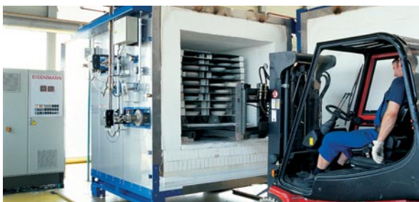
Simple: chamber kiln with manual loading for small series
