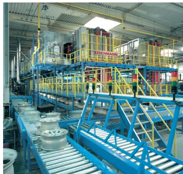
Roller-type ageing oven for aluminum wheels
