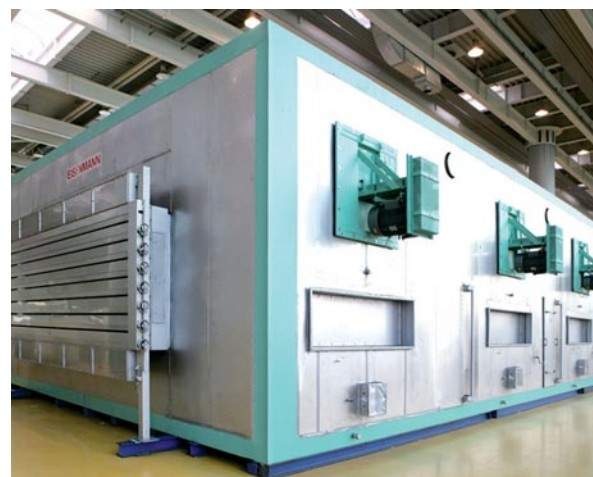
Oxidation oven for PAN fibers for producing carbon fibers
