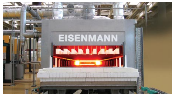
Tunnel kiln for continuous operation
