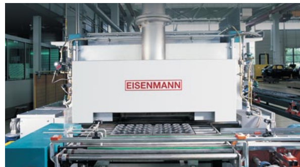
Furnace for sinter metals
