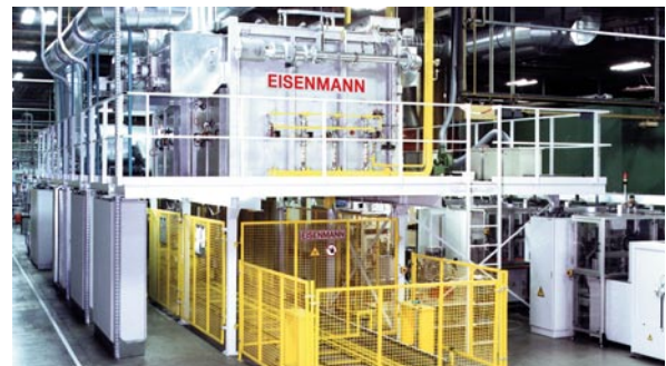
Lift-bottom kiln for automated batch operation
