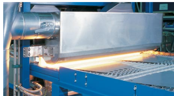
Near-infrared dryer for flat material
