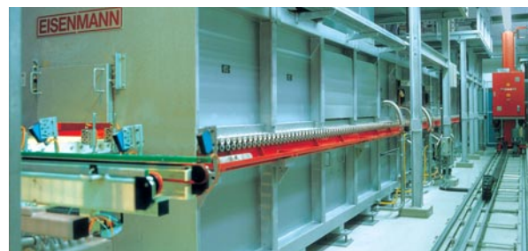
Complex: fully automated roller-type kiln for high throughput
