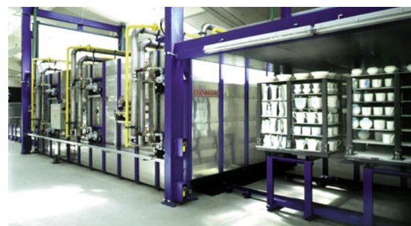
Lift-bottom kiln for porcelain
