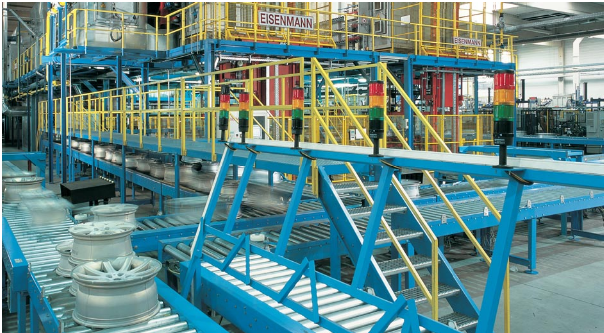
Fig. 3: Mirrored arrangement of heat treatment plants for car wheels with workpieces delivered via roller conveyors
