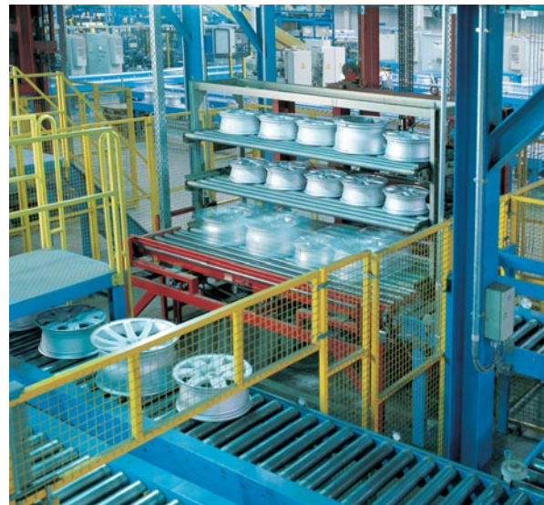
Fig. 1: Lifting station feeding the annealing furnace in an all-automatic roller plant for aluminum wheels
