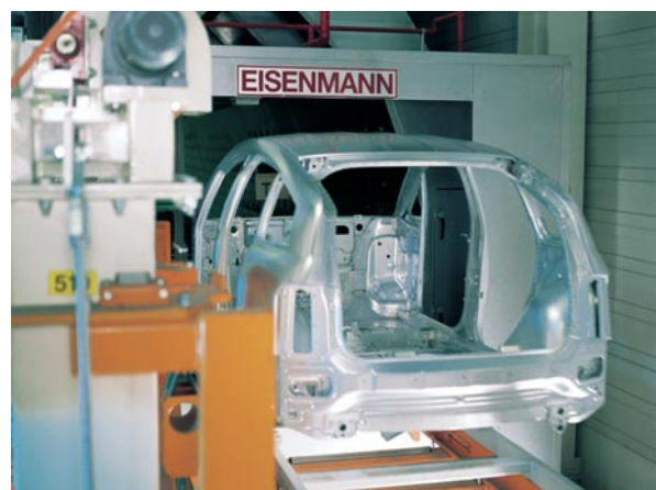
Fig. 11: Inlet of the ageing furnace for aluminum bodies mounted on skids
