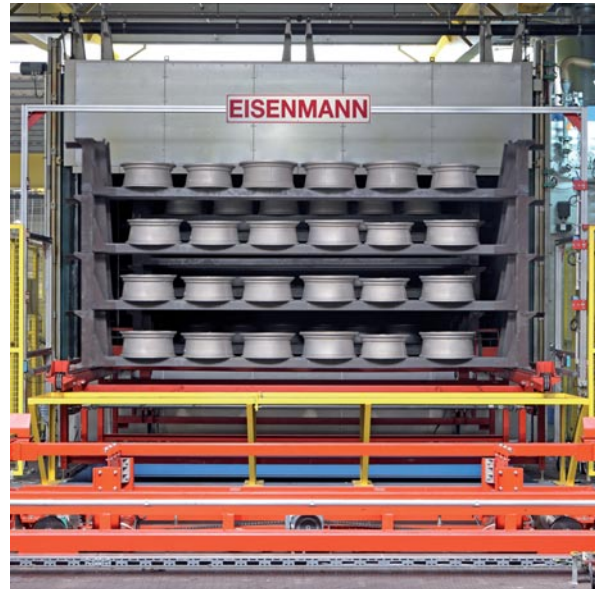
Fig. 7: Outlet of the ageing furnace (push-through plant)
